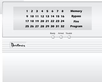
The **P832-16(Z)** and **P832-32(Z)** Keypads are available for applications with more than 8 zones. The functions explained in this manual are the same for all three LED keypad types.
